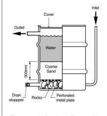
Figure 3. A simple upflow rapid sand filter (Heber, 1985)
