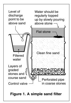
of fine sand. For the filter to perform well there should be no sudden changes in the flow rate and the water should not be very turbid (cloudy with suspended solids), or the filter will quickly become blocked. Good slow sand filters can produce good quality drinking-water.
