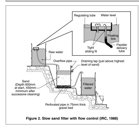
When a slow sand filter is first started, water should be added from below so that it rises through the sand, pushing out the air. If water is added at the top, some air is likely to become trapped between the sand particles, adversely affecting the subsequent performance of the filter.
